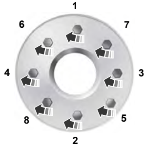
8-lug nut torque sequence
